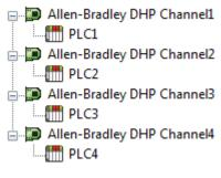
🖃 🐌 Allen-Bradley DHP Channel1 Each device has now been defined under its own channel. In this configuration, a single path of execution is dedicated to the task of 📥 顶 Allen-Bradley DHP Channel2 gathering data from each device. If the application has 100 or fewer channels, it can be optimized as shown here.
